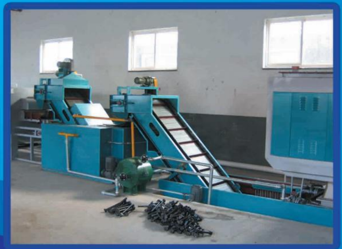
AUTOMATIC HEAT TREATMENT LINE
